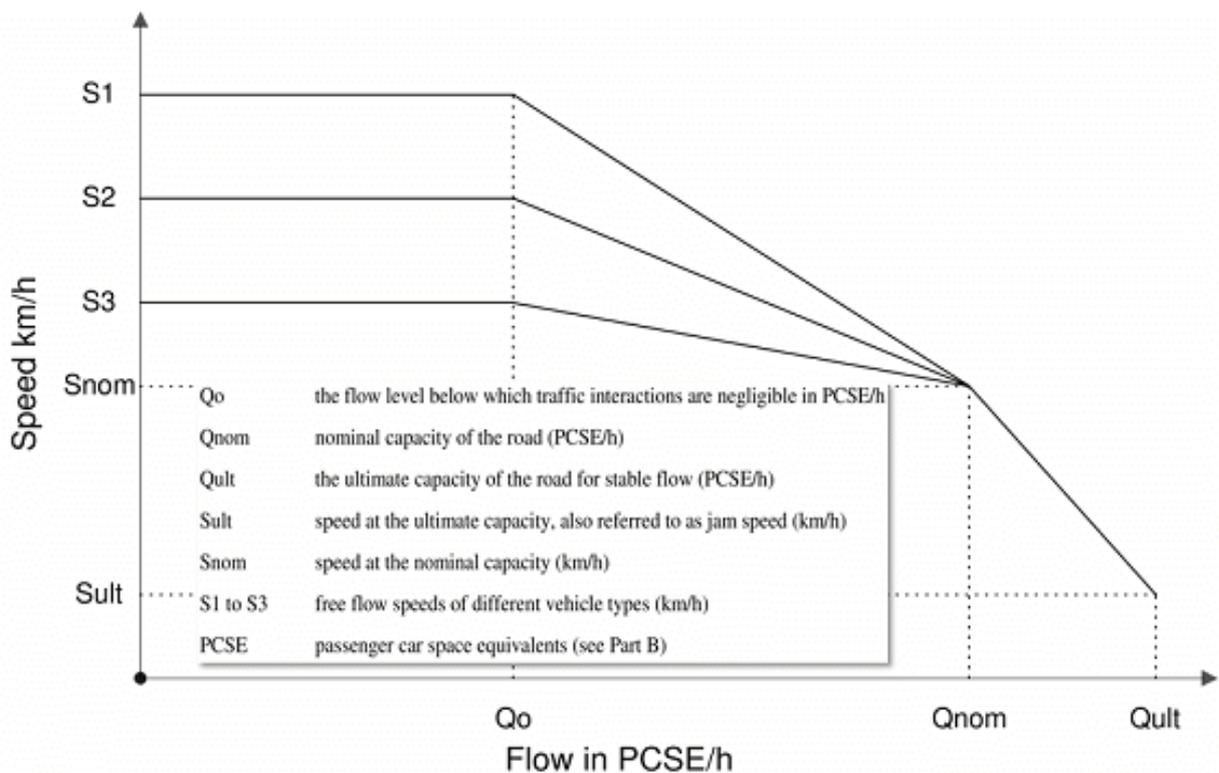
Figure 3. The Characteristic speed in HDM-4
