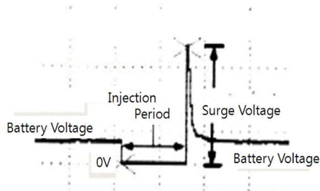
Figure 6. The electric signal of injector
